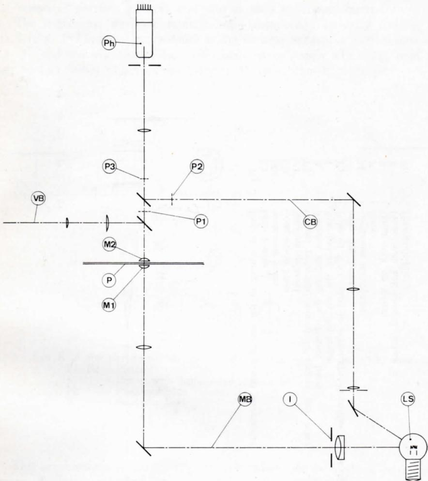
Fig. 1 - The original iris photometer, adapted from EICHNER et al. (1947).
