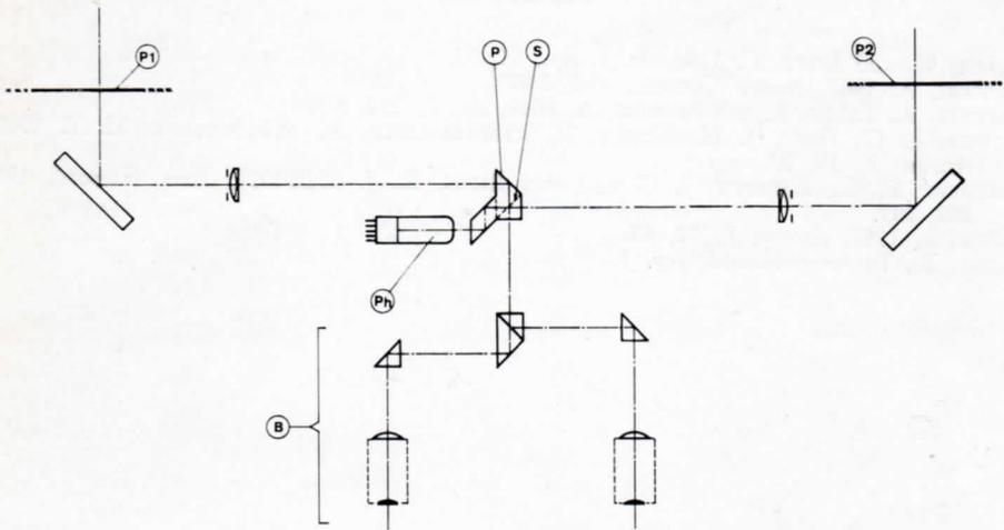
Fig. 3 - Part B of the photometer, included in the viewing optic of the blink comparator.
